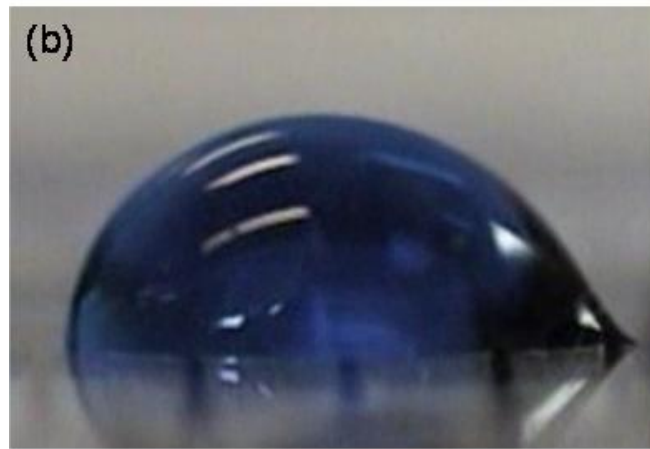
Supplementary Figure S2 a Schematic and b picture of contact angles on actuated ( \theta_{adv} ) and non-actuated ( \theta_{rec} ) electrodes. In this work, the minimum and maximum contact angles were \theta_{adv} = 68^\circ and \theta_{rec} = 115^\circ , respectively. Note that the picture in b does not reflect these values.
