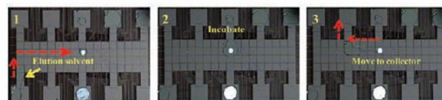
Figure 2. Frames from a movie (left-to-right) depicting the four-step digital microfluidic solid-phase extraction procedure. In (a), a PPM disc is activated by dispensing a 5 \mu\text{L} droplet (frame 1) of activation solvent and driving it onto the monolith. After incubation (frame 2), the droplet is moved away to the waste reservoir (frame 3). Similar steps are repeated for PPM equilibration (not shown), followed by sample loading (b), PPM washing (c), and sample elution (d).
