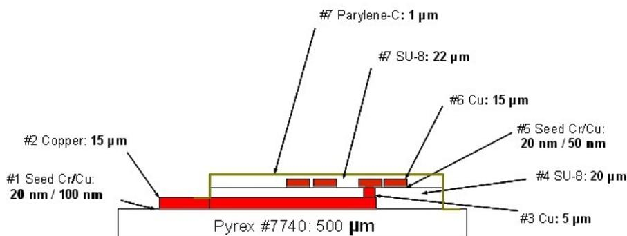
**Figure S1:** Side-view schematic of microcoil. The completed device is formed from seven layers with multiple fabrication steps required for each layer. To increase inductance, multiple turns are used, which required means to form an electrical a cross-over with reasonable size and stability.
