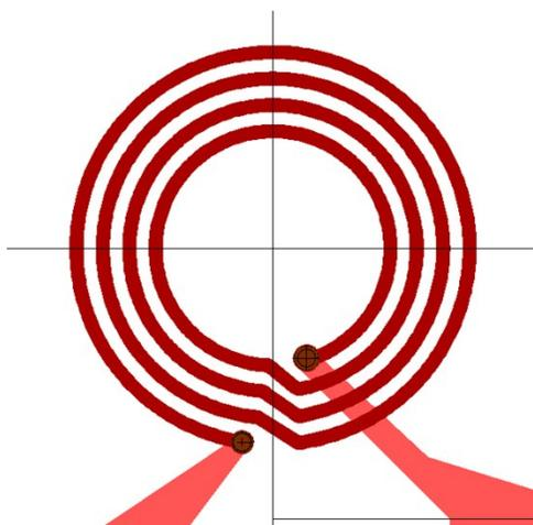
**Figure S2:** Top-view schematic of microcoil. The inner diameter is 500 μm, the outer diameter is 920 μm, the wire width and the gap between wires is 30 μm.
