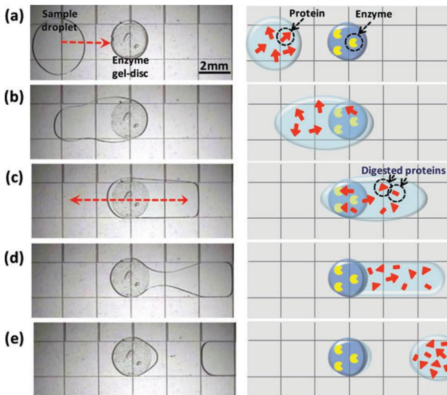
**Figure 2.** Hydrogel proteolytic enzyme microreactors. A series of images from a movie (left) and a schematic (right) depicts a typical digestion in a 2-mm-diameter gel disc on a DMF device. A 2  $\mu$ L droplet containing a proteomic sample is delivered to the gel (a and b), actively incubated (c), dispensed from the gel (d), and then isolated (e). The gel disc contains a suspension of 10- $\mu$ m-diameter beads to make it visible.
