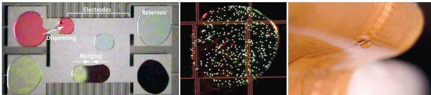
**Digital microfluidics for laboratory miniaturization.** (Left) By applying a sequence of electrical pulses, droplets can be made to move, merge, and dispense on an array of electrodes (these aqueous droplets contain colored dyes and have volumes of 70 nl). (Middle) A very low fluorescence background is useful in
