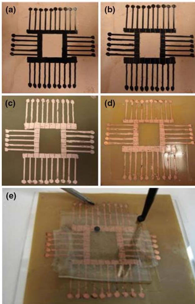
**Fig. 1** Fabrication process. **a** Design is drawn with a permanent marker. **b** A razor blade is used to form gaps between electrodes. **c** Copper is etched in ferric chloride solution and ink is removed using an acetone dampened wipe. **d** Saran<sup>TM</sup> wrap is applied to device surface and treated with Rain-x<sup>®</sup>. **e** Picture of assembled two-plate device. A similar procedure is used to fabricate devices from compact disk substrates
