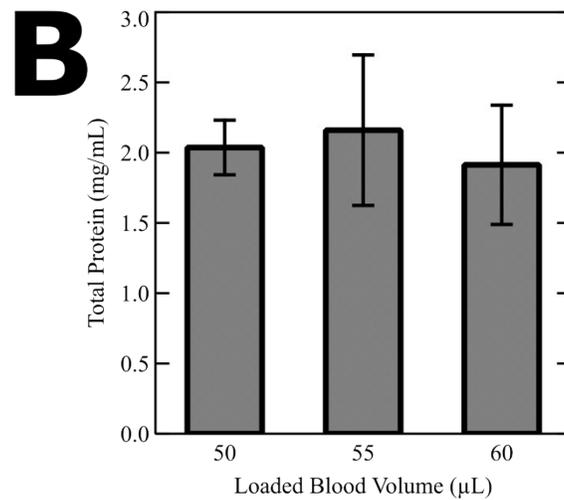
**Supplementary Figure S2.** World-to-chip interface and sample loading. (A) Frames from supplementary movie M1 (left-to-right) demonstrating a whole blood droplet “dabbed” from a finger onto the SM. (B) Plot comparing the total protein measured in diluted plasma droplets generated from different volumes of blood loaded onto the device. Error bars represent  $\pm 1$  standard deviation from  $n = 3$  replicates per condition.
