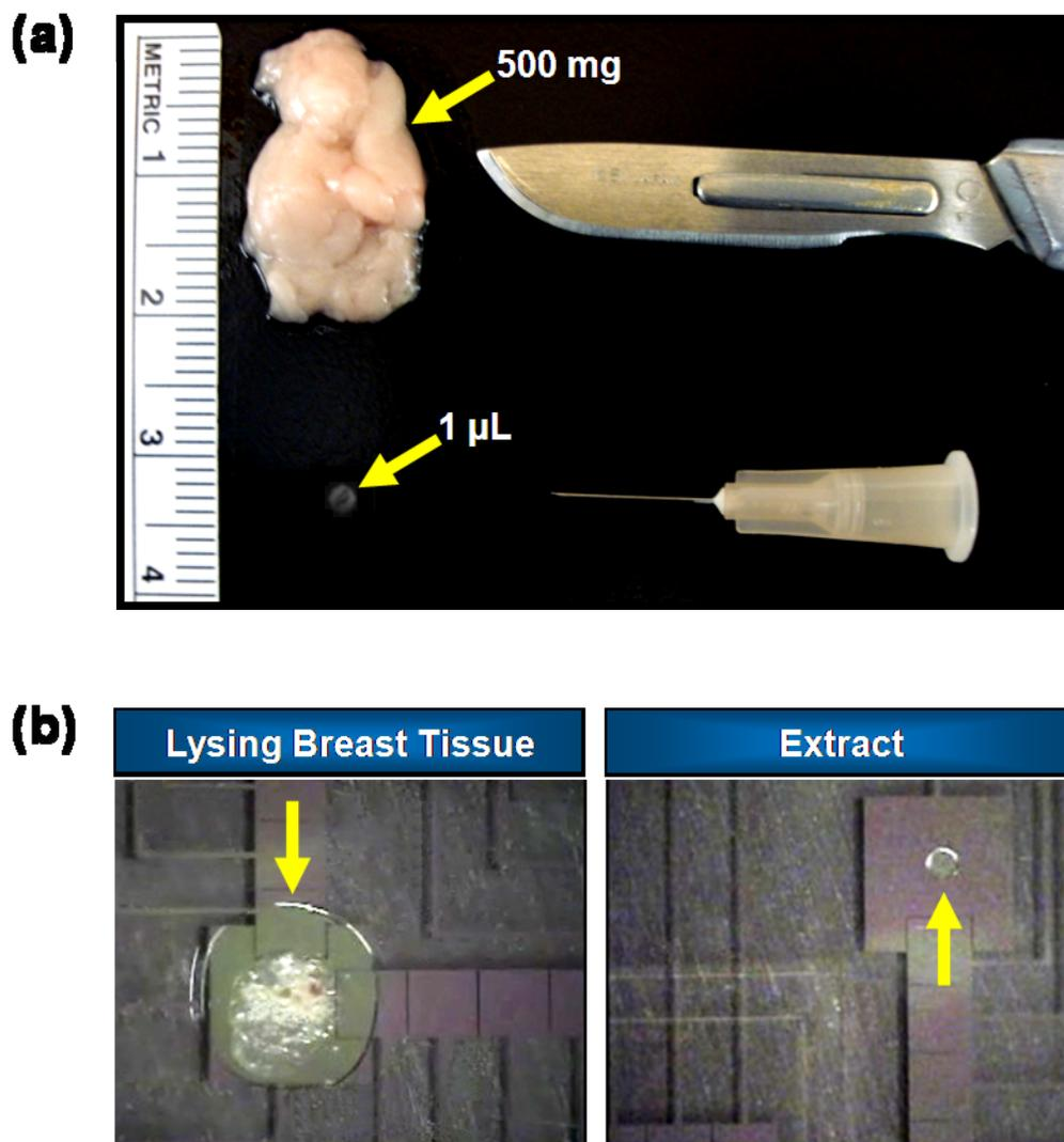
**Figure 1S: Reduction in Sample Volume.** (a) Picture of 500 mg of breast tissue collected by incisional biopsy (representing the sample size required for conventional analysis methods) compared to a 1  $\mu$ l microaspirate collected using a 30 ga. needle (representing the sample size used with the new method). (b) Pictures of breast tissue microaspirate (1  $\mu$ l) being lysed on the DMF device and of the dried estrogen extracted from it.
